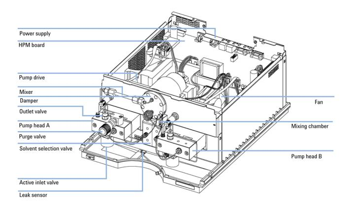
The binary pump is based on a two-channel, dual-piston in-series design which comprises all essential functions that a solvent delivery system has to fulfill. Metering of solvent and delivery to the high-pressure side are performed by two pump assemblies which can generate pressure up to 400 bar.
