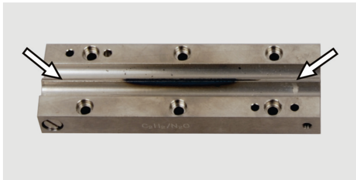
Fig. 54 Spacers inserted in burner jaws
