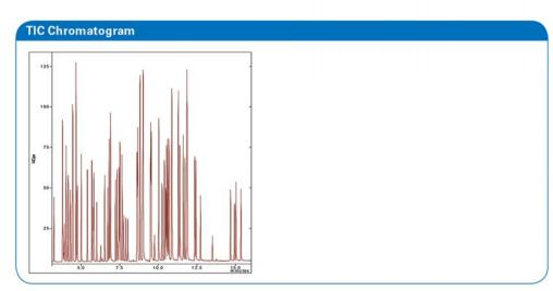
TIC chromatogram of a 5 mL water sample containing 84 VOCs at 10 µg/L (ppb) by US EPA Method 524.3
